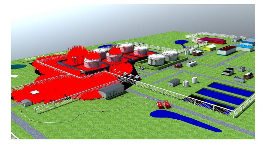
• Three foam attack using sublayer method of extinguishing fires in the tank Nº4 were organized in the period of time from 20.00 on 23<sup>rd</sup> August, 2009 to 04.00 on 24<sup>th</sup> August, 2009. This made it possible to practically stop the burning and to prevent an explosion in the tank Nº4.
